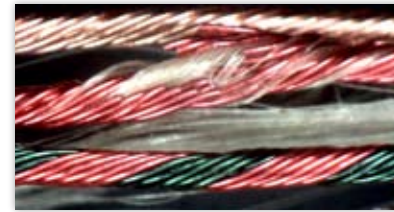
Cable breakage after repeated bending
